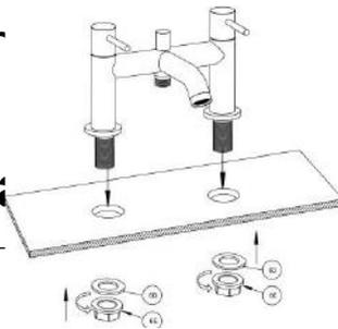
Remove the rubber gaskets(6D) and locknuts(6E) from the Legs.
